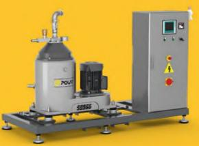
Centrifugal systems operate in by-pass mode with a collecting tank. Experience has shown that good oil quality is obtained if the tank has a capacity equal to 20 times the hourly flow rate of the separator. A purifier separates sludge and water from the oil. Water is continuously discharged from the bowl. The sludge accumulated in the sludge space in both a purifier and a clarifier is intermittently discharged
